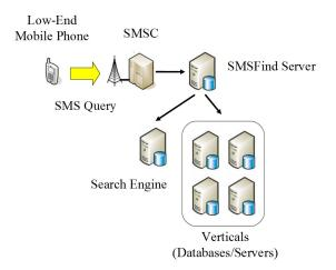
Figure 1: System architecture
